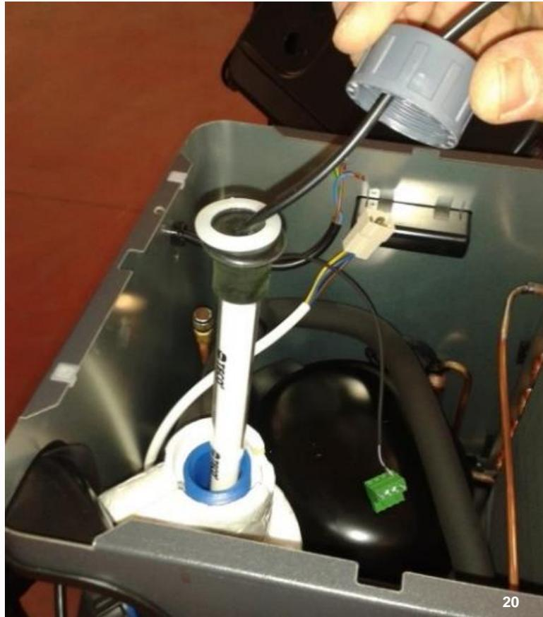
*Disconnect the heater connector (img.22)*
